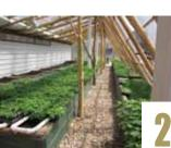
This passive solar green house was designed to use as little fossil fuel energy as possible. The 56° angle of the southern face and the building's orientation at 2° east of south provide maximum solar gain during
